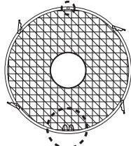
2. Press down all the Buckles to fasten the Front Guard with the Rear Guard. At the Screw Holes, tighten the separated screw and nut.
