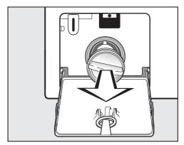
■ Remove the drain filter completely.
