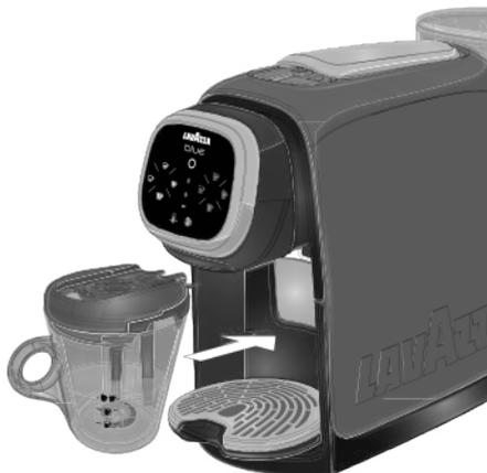
**4** Press the **LATTE MACCHIATO** button ☕ to start the cleaning cycle.
