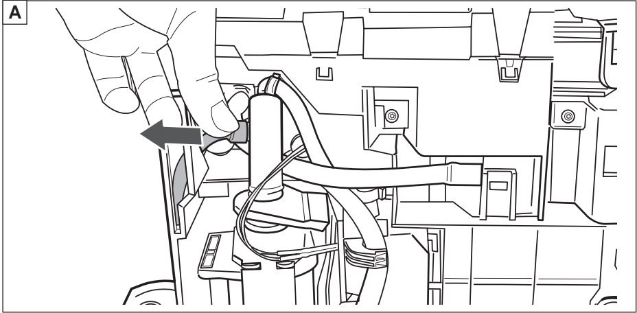
Figure A: disconnect the hose connecting the self-priming valve (pump).
